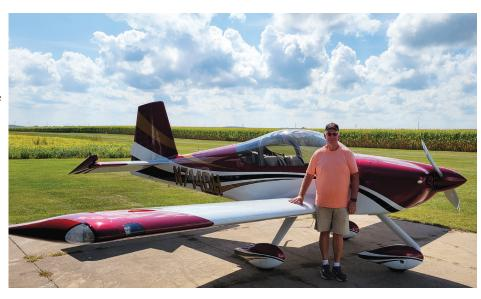
Harm finished building his Vans RV-14A with a 210 HP engine in fall of 2021. "The most challenging part of the build were the fuel tanks," shared Harm. "Each rivet in the tank needed to be sealed so fuel wouldn't leak out. A messy and time-consuming process."
